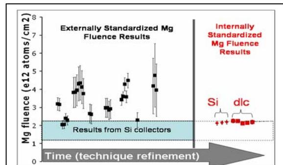
Fig. 1. Mg Fluences, ordered by run date. Blue bar represents the range of 28 analyses of Si collectors; the black data are individual analyses of dlc collectors. Both were made relative to external standards. Red points are for analyses standardized internally, by implanting flight samples with <sup>25</sup>Mg. Here, fluences from DLC and Si collectors (as marked) agree.
