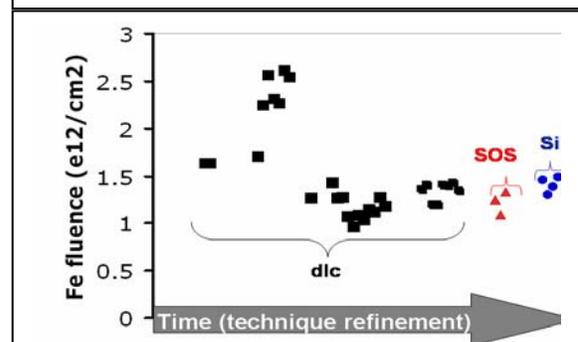
Fig. 2. Fe Fluences ordered by run date. Tightly controlling analytical procedures gave progressively more consistent results both for the same material and for different materials (Si, SOS, and dlc). Internal standardization was not necessary. Statistical error for individual analyses are about the size of the symbol.
