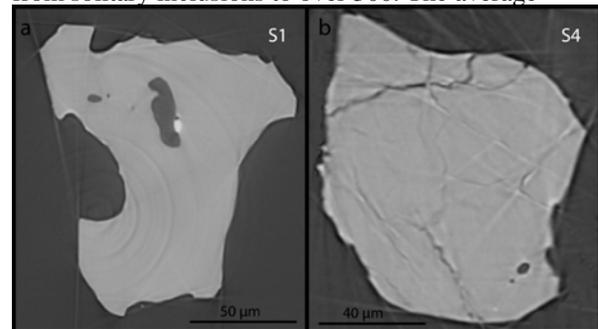
Fig. 1. Virtual slices through microtomograms of chromite grains with inclusions and different degrees of fracturing. Also shown are the previously assigned shock stages (S1-S6) of the chondrites that the chromite grains derive from. a) Grain with polymineralic inclusion of silicate and metal/troilite extracted from H6 chondrite Kernouvé. Also note the absence of fractures. b) Relatively fractured grain with two small inclusions in the lower right corner, extracted from L5 chondrite Farmington.
