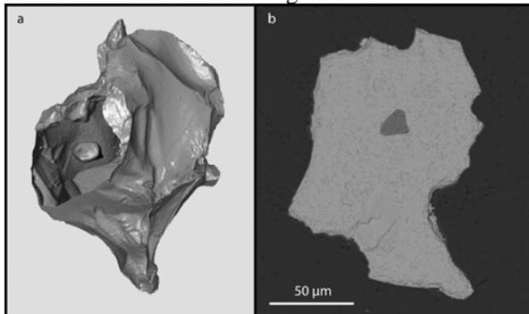
Fig. 2. a) 3-D rendered image of chromite grain extracted from H6 chondrite Kernouvé with inclusion of Ca-poor pyroxene. b) SEM backscatter image of the same chromite grain, now mounted in epoxy and polished down to display the inclusion.
