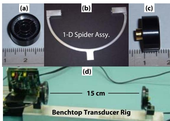
Fig. 3: (a, c) SASA ultrasonic transducers have good acoustic impedance match to the martian atmosphere. (b) The aluminum spider assembly has low thermal expansion, maintaining a constant distance between transducers during operations. (d) SASA has been tested in STP and static vacuum chamber conditions.
