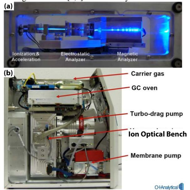
Fig. 2: (a) RAMS Ion-Optical bench with Ion-Cam CCD detector on right. (b) Unmodified commercial unit from OI Analytical. The ASTRA flight unit uses a ion pump and eliminates the GC oven, allowing rapid sampling, but the Ion Optical Bench is identical.
