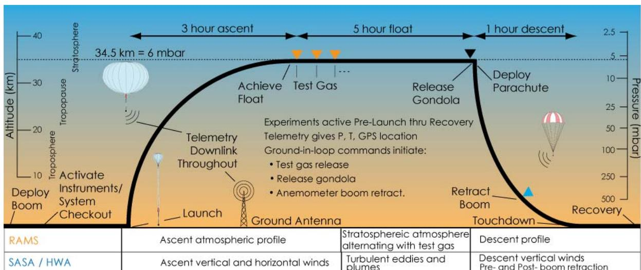
Fig. 1: ASTRA launches with all instruments activated, recording ascent and descent profiles as well as the at-float environment. All data is recorded to on-board solid-state memory, with data snapshots transmitted to the ground station in real-time. All instruments are shut down following boom retraction but before touchdown.
