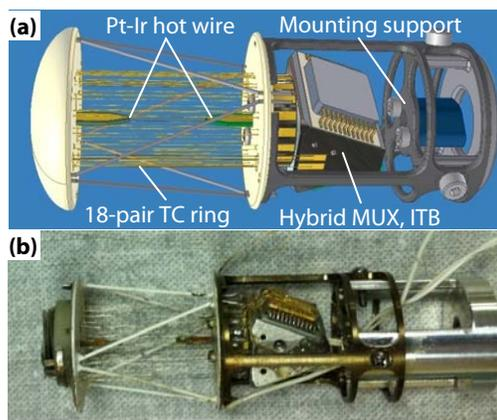
Fig. 4: (a) HWA schematic showing strut assembly with 18 thermocouple pairs in a ring (yellow) for wind-direction determination, Pt-Ir hot wire (center of TC ring) for wind-speed, the hybrid MUX and isothermal block, and mounting support. (b) completed engineering model. The HWA is 3.5 inches long.
