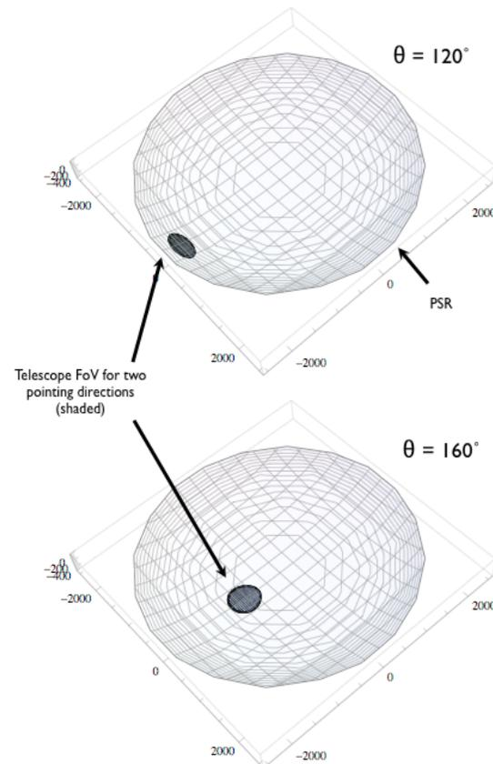
Figure 1: Crater Geometry Example. Two examples of the ellipsoidal crater model showing the projected neutron telescope field-of-view. The telescope is located at crater center with viewing angles as shown (relative to zenith).
