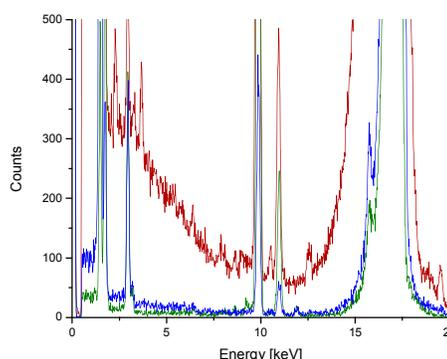
Figure 1: TXRF spectra of Genesis sample SAP 50719 before acid cleaning (red), after HCl only cleaning (green), and HF/HCl cleaning (blue).
