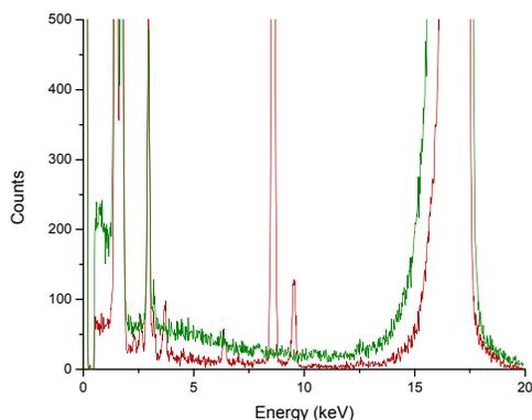
Figure 3: TXRF spectrum of Genesis sample SOS 60326 before acid cleaning (red), after HCl cleaning (green).
