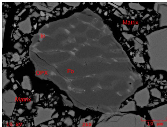
Figure 1. BSE image of 'Mg-Fragment 1' in 60016,93, composed of Fo<sub>98</sub> olivine (Fig. 2a), enstatitic pyroxene (Fig. 2b) and an interstitial component (In).
