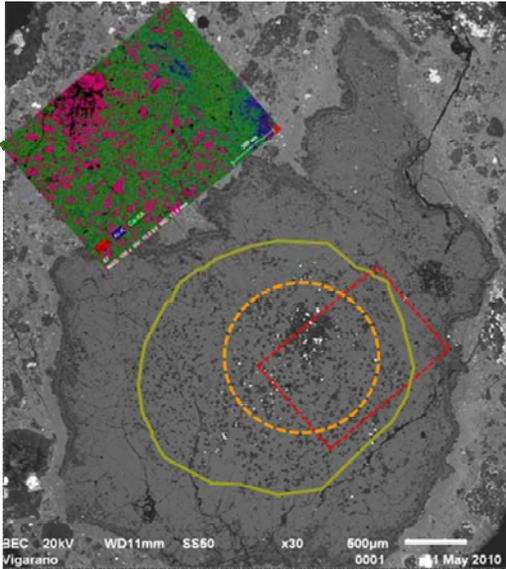
Fig. 1. BSE image of type B Vigarano CAI #1; A combined elemental mosaic of the inset rectangle Al (blue)-Mg(Red)-Ca(green) is shown in the upper left corner. The dashed circle represents the area that has been considered as the core which is rich in spinels, while the minerals present in the region outside the solid line (devoid of spinels) have been considered as minerals present in the boundary of CAI.
