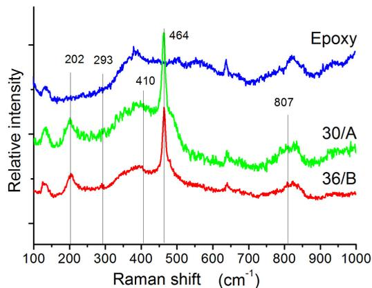
**Figure 4.** Representative spectra of the epoxy coating, and of the 36/A and 30/B quartz grains.
