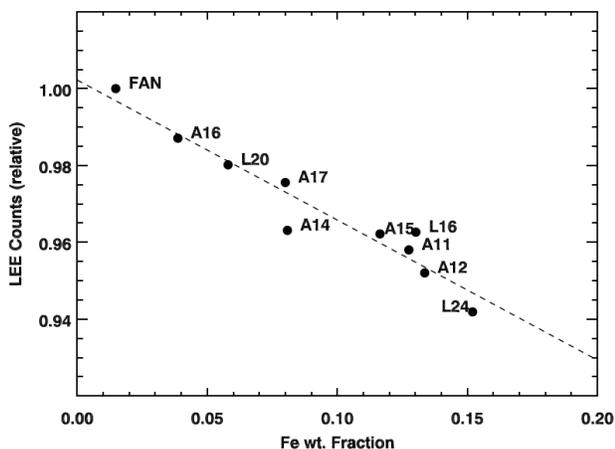
**Figure 1.** Modeled LEE epithermal neutron count rate versus Fe content for various returned lunar soils (adapted from [3]). Relative count rates are calculated for the LP <sup>3</sup>He neutron sensors. The count rates are anticorrelated with Fe content. The anticorrelation is confirmed with LP orbital data [3,9].
