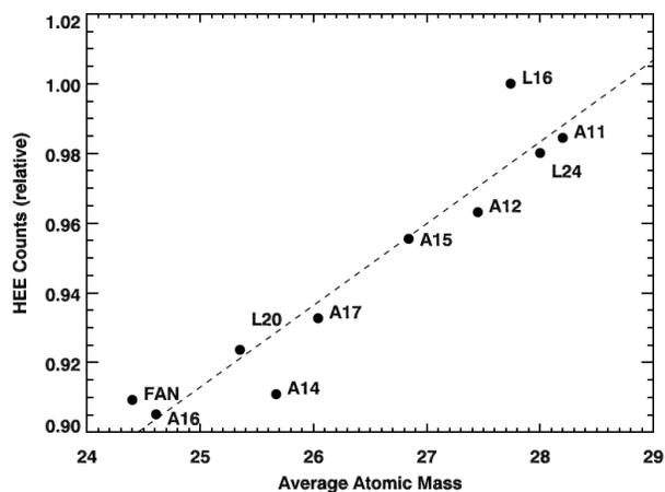
**Figure 2.** Modeled HEE ( $E_n > 1$  keV) epithermal neutron count rate versus average atomic mass for returned lunar soils. Relative count rates are calculated for the LP <sup>3</sup>He neutron sensors. In contrast to LEE neutrons, HEE neutrons show a positive correlation that is similar to the behavior of fast neutrons.
