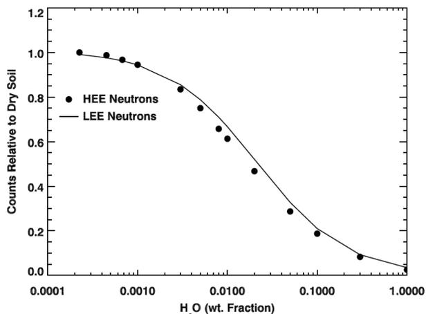
**Figure 3.** Modeled epithermal neutron count rate ratio (dry/wet) versus water equivalent hydrogen content for lunar ferroan anorthosite soils. HEE neutrons from <sup>3</sup>He sensors are circles. LP LEE-dominated neutrons are the solid line from fit of [3].
