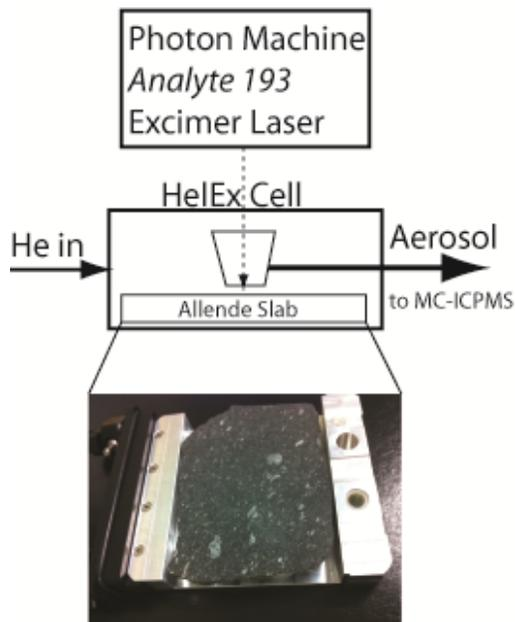
**Figure 2.** Photograph of modified sample holder for PhotonMachines HelEx cell. Allende slab measuring 8 cm x 10.5 cm x 0.5 cm is sitting in sample holder for reference.
