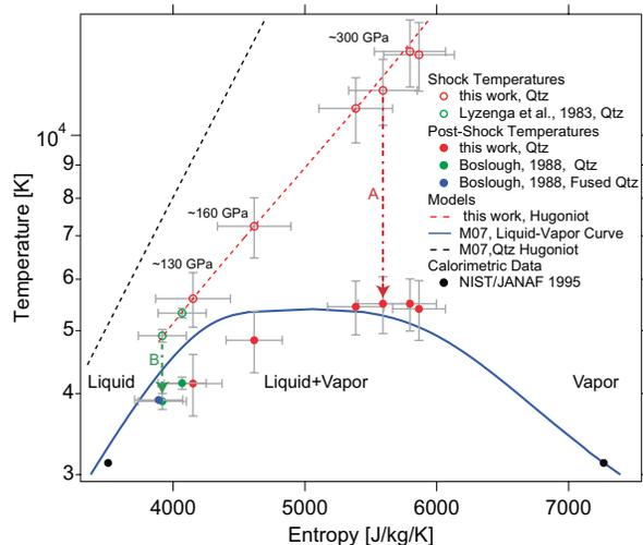
**Figure 2:** Data from Fig. 1 on a temperature-entropy phase diagram for silica. The shock wave rapidly compresses the silica, increasing the entropy. Because decompression is isentropic, paths A and B are vertical lines.
