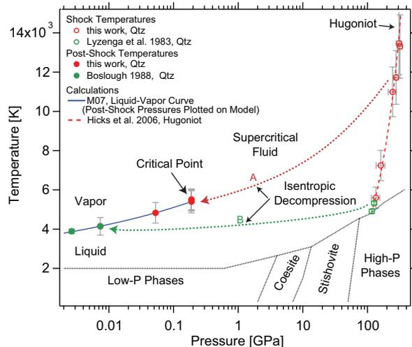
**Figure 1:** Temperature-pressure phase diagram of silica. In each experiment, quartz is shocked to a fluid state on the Hugoniot (open symbols) and then decompresses isentropically to the liquid-vapor curve (filled symbols) along schematic paths A and B, starting at  $\sim 310$  and  $\sim 120$  GPa.
