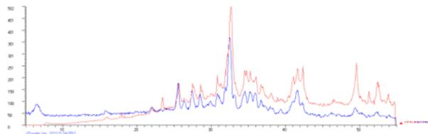
Figure 2. Comparison of XRD data from Terra (blue) and XTRA (red) using a Lunar soil (#14163). Differences in peak relative intensities are due to the sensitivity to grain size with the XTRA breadboard.
