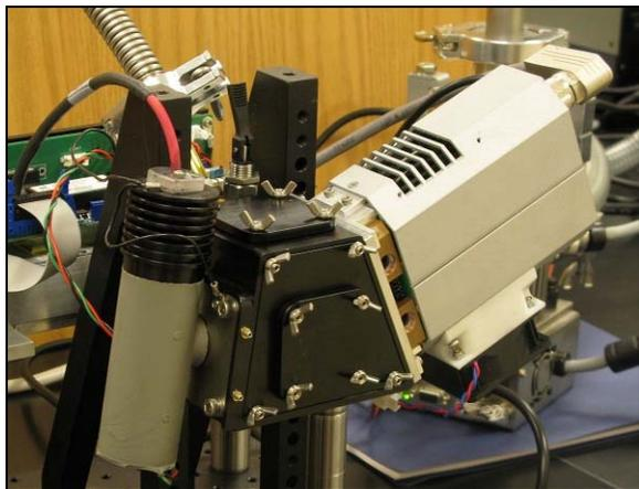
Figure 1. XTRA breadboard built with commercial components to test the geometry and operation under vacuum. Left to right: X-ray tube, vacuum chamber, CCD camera.
