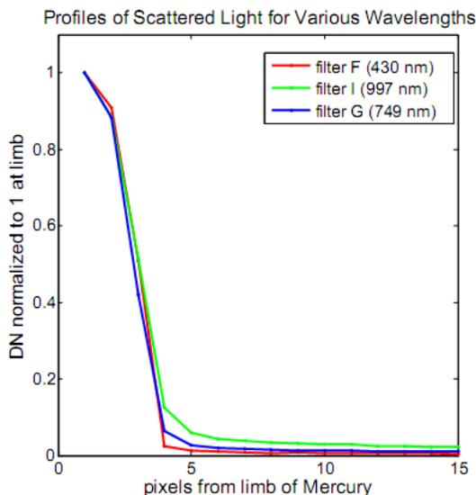
**Figure 1.** Profiles of Scattered Light for Various Wavelengths. Plot illustrates that scattered light increases for longer wavelengths.
