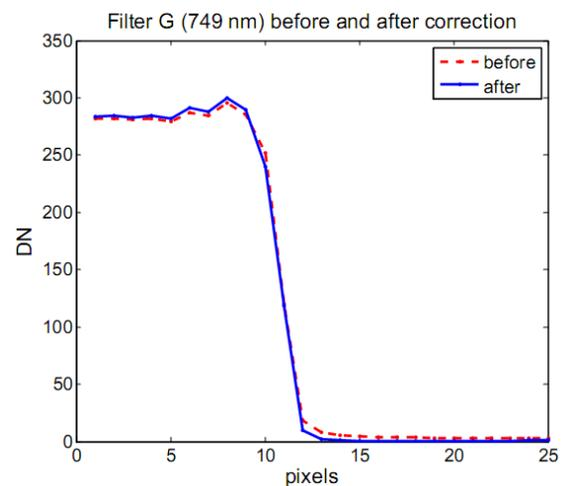
**Figure 2.** Profiles across the limb of Mercury before and after the deconvolution, for filter G. Conceptually, the deconvolution moves light scattered in space back onto the disk of Mercury.
