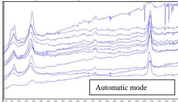
The automatic method takes longer times but implies risks of damage in the thermolabile samples, however, it has shown to be a more accurate procedure, being able to detect mineral species that were not detected by visual exploration in brilliant samples.
