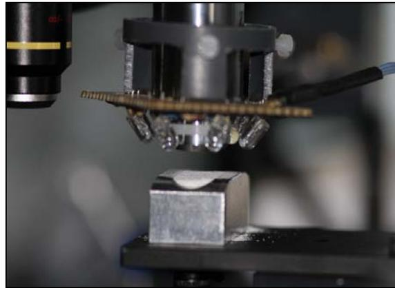
In the first case, the probe head goes over the sample along evenly spaced steps and takes spectra at each point. In the second one, the selection of the targets on the sample is made based on images and an observer and the experience choose the targets of analysis.
