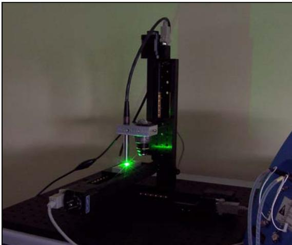
With the aim of evaluating the precision of the system and the effects on the sample due to the laser radiation, the system has a camera to verify the spot's posi-
