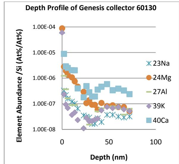
**Figure 6.** Simultaneous depth profiles into silicon sample 60130 obtained after further HCl cleaning of the surface.
