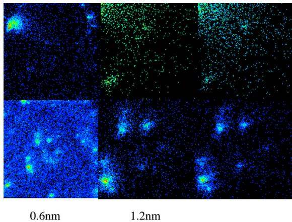
**Figure 5.** Successive elemental maps (Al first row, Ca second row) with depth into the surface.
