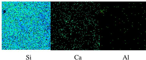
**Figure 2. Adjacent 200micrometer area showing little contamination on the surface.**
