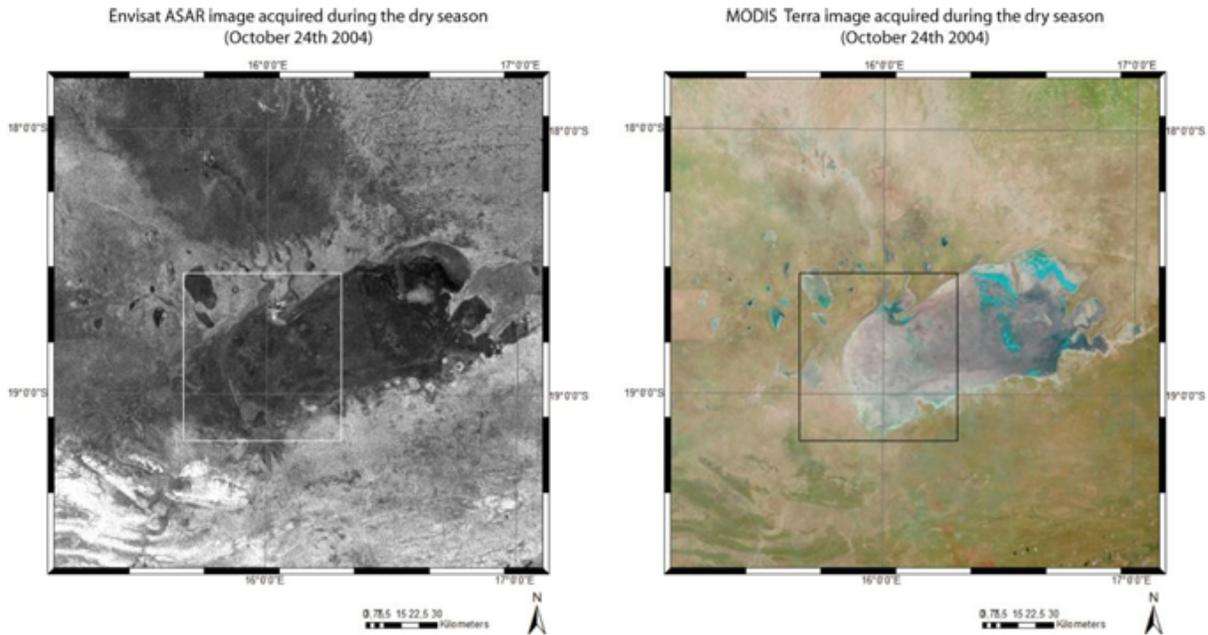
Figure 2: Observation of the Etosha region in October 2004 during the dry season. Left: Envisat ASAR image. Both liquid-covered and liquid-free portions of the pans are darker than their surroundings. Data provided by the European Space Agency ©ESA 2004, ESA ©; right: RGB MODIS color composite provided by the National Aeronautics and Space Agency NASA/GSFC, MODIS Rapid Response.
