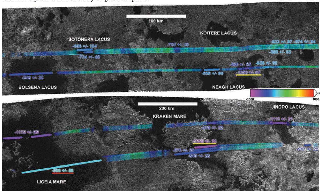
Figure 1: High resolution SARTopo of parts of the T16 and T25 RADAR swaths, draped over their associated BIDRs. Transparency gives a crude indication of certainty, being a representation of a function based on SARTopo footprint size and along-track distance from the footprint centre. No geoid correction has been performed on this version.
