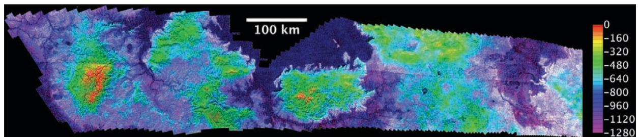
Figure 2: Stereo-derived DTM (courtesy: R. Kirk, USGS Flagstaff) for comparison with T25. No geoid correction has been performed, and the colour scale differs from that of Fig. 1. Absolute elevations are in good agreement with SARTopo, as coarser resolution SARTopo was used to adjust the stereo product. Local variations also appear to be in good agreement, providing cross validation. Further work will be performed to extend the comparison.
