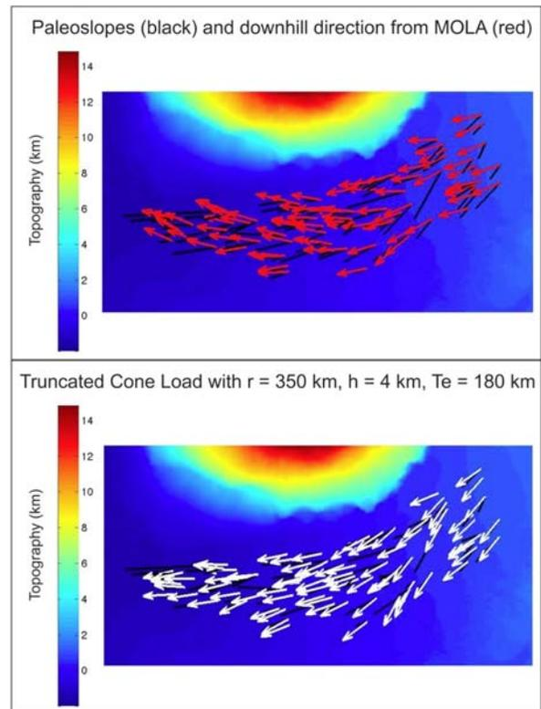
Figure 1. Paleoslope orientations (black lines) connecting the beginning and endpoints of mapped flows. Red arrows show current downhill direction from MOLA. Paleoslopes and predeformation downhill direction (white arrows) from the flexural loading model.
