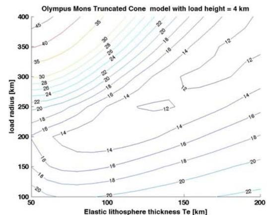
Figure 3. Root-mean-square (r.m.s.) misfits between observed lava flow azimuths and downhill azimuths for a truncated cone load calculated by removing the effects of a loading model from observed topography. Contours are in units of degrees. Model parameters are elastic lithosphere thickness  $T_e$  on the x-axis and load radius on the y-axis. Load radii larger than 400 km were not considered because they would cover the flows that are being used to infer paleoslopes. Load height is 4 km.
