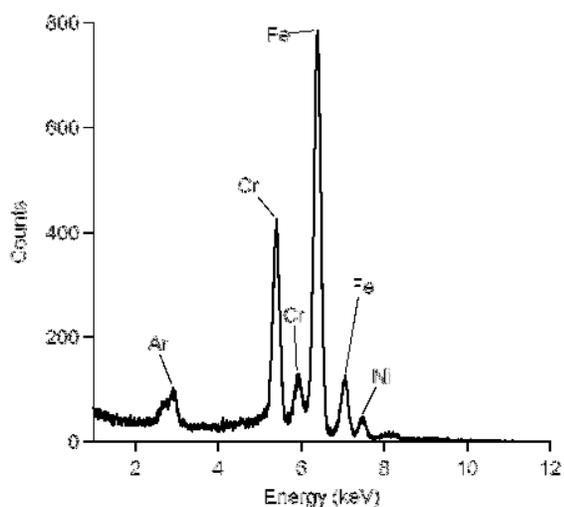
**Figure 3:** Spectrum of stainless sample, acquired with the Micro-XRF breadboard instrument.
