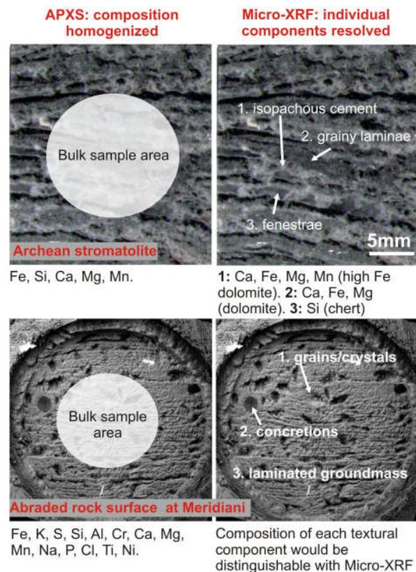
**Figure 1:** Comparison of analyses performed by APXS (left) and Micro-XRF (right). Top: Micro-XRF reveals the composition of important, separate components of an Archean stromatolite. Bottom: Bulk elemental data leaves significant unresolved questions about the geologic history of this martian rock (lower image courtesy Caltech/JPL).
