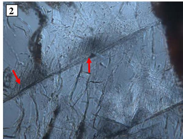
Fig. 2 Feather features (arrows) in quartz, core sample depth 390.1 m, X-pol; image is  $\sim 280 \mu\text{m}$  wide.
