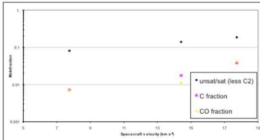
Figure 3: Changes in carbon content as a function of flyby velocity.
