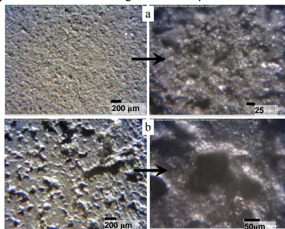
Fig. 3. Microstructure of sintered regolith at 20 wt % Al with (a) 2 wt % Teflon and (b) 7 wt % Teflon.
