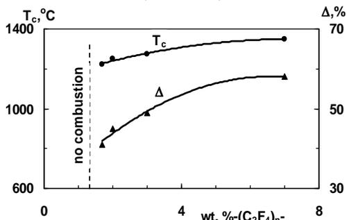
Fig. 2. Combustion temperature and product porosity as a function of Teflon concentration in the mixture.
