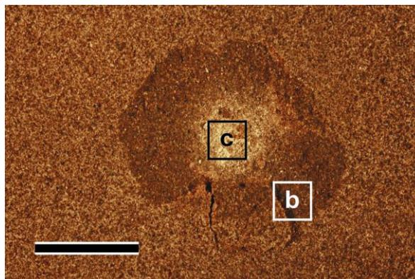
Figure 1. Impact crater and sample positions. The scale-bar represents 1 cm.
