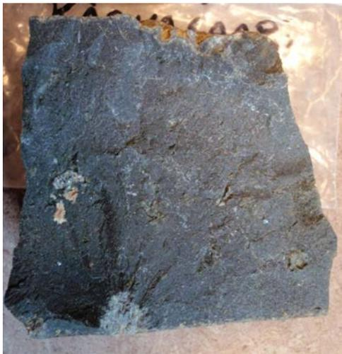
**Fig. 1.** Almost clast free melt rock from Lappajärvi, Finland. The rock piece is 4 cm across.
