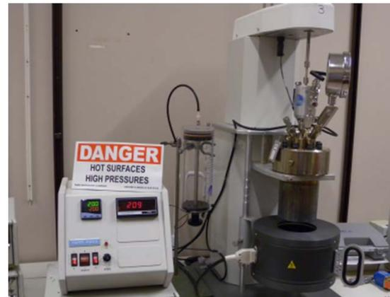
**Fig. 2.** The experimental setup with Parr © titanium reactor.
