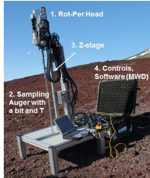
**Figure 1. Components of the IceBreaker Mars Drill. The IceBreaker drill in the University Valley, Antarctica was used to drill 1 meter in ice-cemented ground and collect drill cuttings.**
