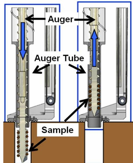
Figure 5. Sample acquisition and storage within the Auger Tube.
