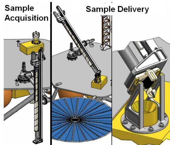
Figure 4. 3 DOF boom enabled sample delivery.
