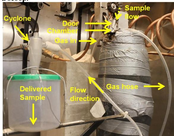
Figure 3. Pneumatic sample transfer.
