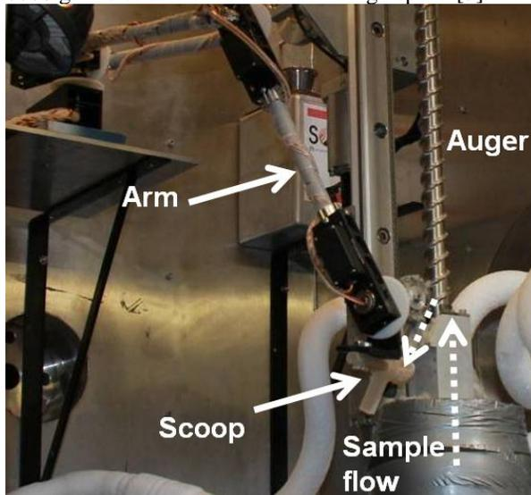
Figure 2. Sample transfer using a robotic arm with a scoop.
