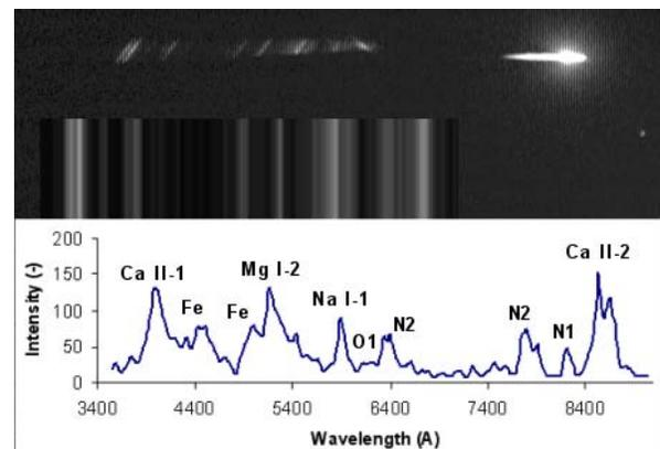
Figure 3. Raw and processed emission spectrum of the SPMN140111 Comae Berenidids fireball.
