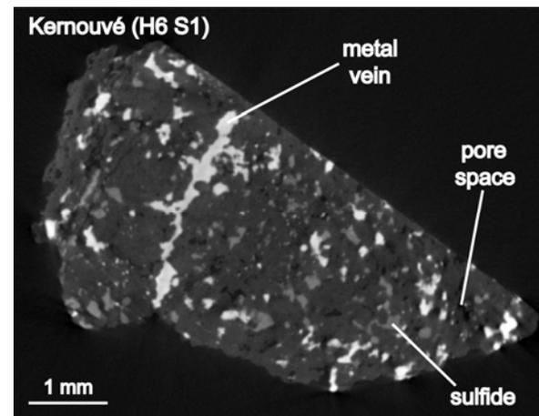
**Figure 1.** A  $\mu$ CT slice of the AMNH 470 Kernouvé (H6, S1) chondrite sample. A metallic vein and intragranular porosity can readily be imaged with resolutions of  $\sim 11 \mu\text{m}/\text{voxel}$ .
