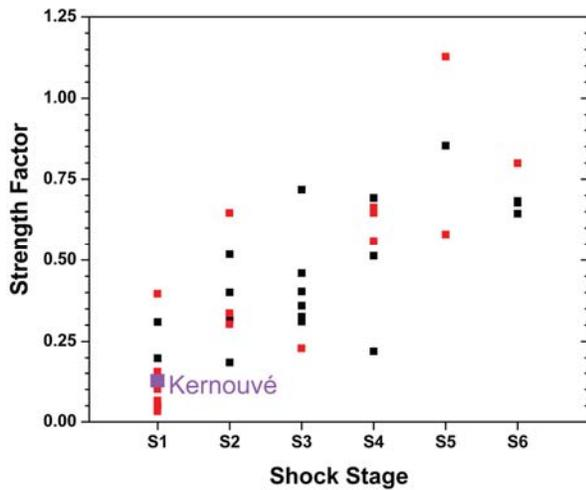
**Figure 2.** Degree of compaction, as given by the strength factor determined by collective orientation of metal grains in chondritic samples [12], versus shock stage. Kernouvé is not only mildly shocked, but also poorly compacted. Data in black [12] incorporated only L chondrites; new data (red symbols and Kernouvé) incorporating H and LL chondrites, demonstrate that the scheme holds for chondrites other than L.
