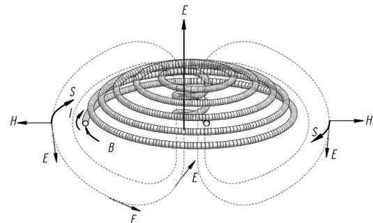
Fig. 2 shows the momentary arrangement of the electromagnetic field created by the propulsion system by the application of solenoid cable with  $I$  current
