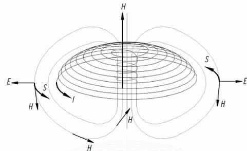
Fig. 1 shows the momentary arrangement of the electromagnetic field created by the propulsion system by the application of straight cable with  $I$  current
