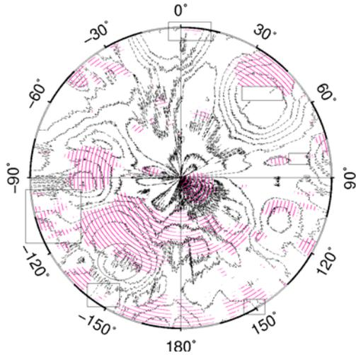
Fig.1 Unaccessible communication region (red and pink line) of the lunar rover from the Earth to the Moon in the lunar south polar based on DEM of Kaguya/SELENE, between tracking stations and lunar rover, the top is Shanghai tracking station, the below is Chinese Antarctic Great Wall station. The black box and circle describe the region that communication condition improved.
