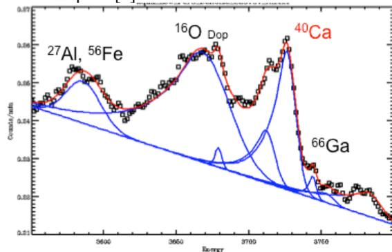
Fig. 5. Many peaks near and below the 3737 keV peak used for calcium. Sources of larger peaks are given [6].
