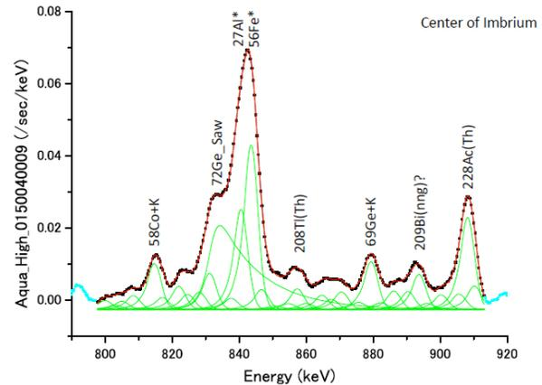
Fig. 6. There are many peaks that overlap from 800 to 910 keV, making it hard to use these gamma rays. The big peak at 843 keV is from Al, and the peak at 847 keV from Fe is weak. Both of those peaks are on a wide ‘sawtooth’ feature from Ge starting at 834 keV.
