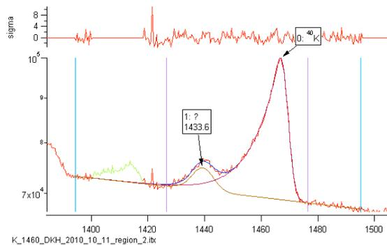
Fig. 1. Peak for potassium at 1461 keV. The peak at 1434 keV is from excited <sup>52</sup>Cr, mainly made in Fe.
