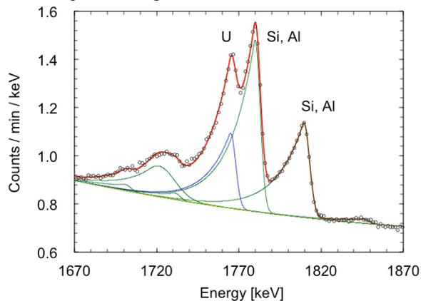
Fig. 4. Spectrum around the 1764 keV peak used for U (blue). The peak at 1779 keV is made by  $^{28}\text{Si}(n,\gamma)$  reactions and the decay of  $^{28}\text{Al}$  made in structural Al.
