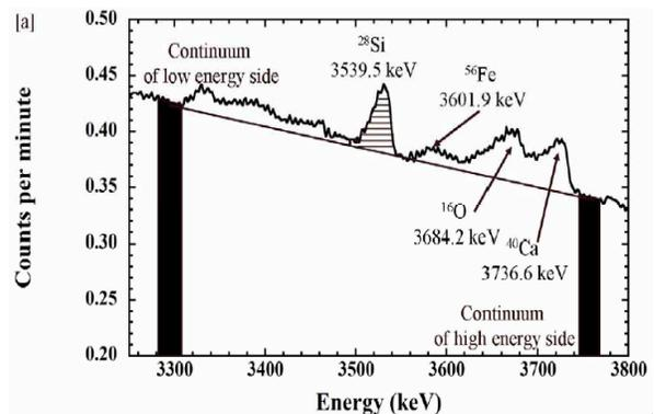
Fig. 3. KGRS peaks around the 3539 keV gamma ray used for Si.
