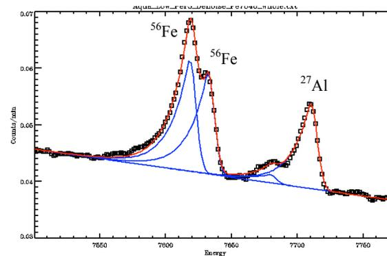
Fig. 2. Peaks for the iron neutron-capture doublet at 7631 and 7645 keV (left) and the Al neutron-capture gamma ray at 7724 keV.
