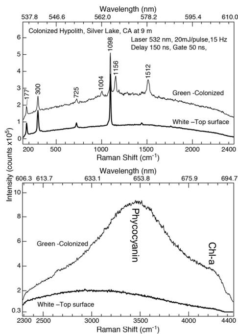
Fig. 2. Combined stand-off TR LINF and Raman spectra of colonized hypolith from Silver Lake, CA. Laser 532 nm, 24 mJ/pulse, gate 50 ns, slit 100  $\mu$ m.
