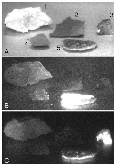
Fig. 1. Photographs of rock samples with 0.1 s exposure time at 2 m distance with gated ICCD camera with (A) White-light illumination; (B) with short life-time LINF (gated 200 ns) and (C) with long-life time LINF (4 ms gate) excited with 532 nm pulsed laser.
