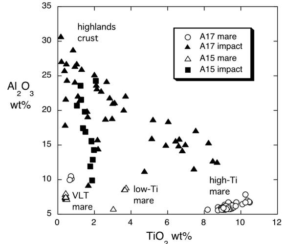
Fig. 1. Plot of Al<sub>2</sub>O<sub>3</sub> vs TiO<sub>2</sub> wt% for 78481 and 15221 regolith spherules.
