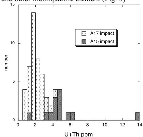
Fig. 2. Histogram of U+Th contents of impact spherules from 78481 and 15221.
