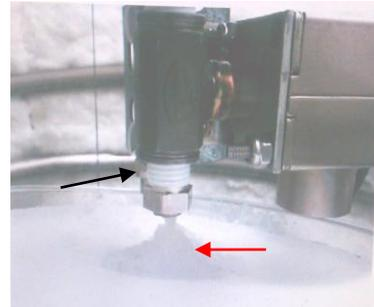
**Figure 3.** Acetylene slurry poured into sample pan (red arrow). Black arrow shows the fiber optic probe behind the output of the solenoid valve.
