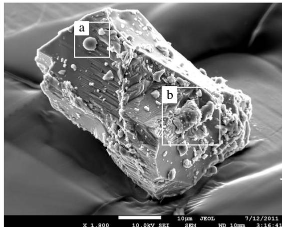
Figure 2: RA-QD02-0116 with abundant adhered objects. (a) DOO and (b) PIC are stuck on the surface.
