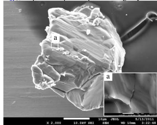
Figure 1: Surface images obtained by SEM of the entire grain RA-QD02-0121. Shock lamellae are developed on olivine substrate. (a) Quenched melt on and along a crack.
