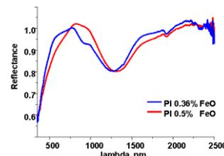
Fig. 1 VIS-NIR plagioclase reflectance spectra (63-125  $\mu\text{m}$  grain size) normalized to 750nm for comparison.
