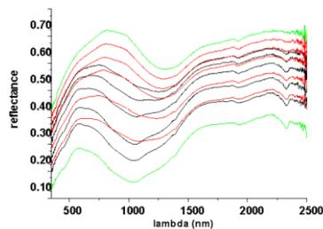
Fig. 5 End-member, iron-rich PI, and Ol-rich mixtures are in green, in black are the real mixture spectra and in red the mixture spectra calculated as simple combination of end-members.
