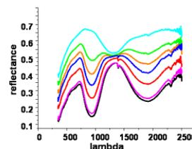
Fig. 2 Ol-free+ iron-rich Pl mixture's reflectance spectra. Pl % increases from black to light blue.
