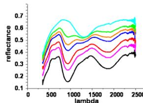
Fig. 3 Ol-poor+ iron-rich Pl mixture's reflectance spectra. Pl % increases from black to light blue.
