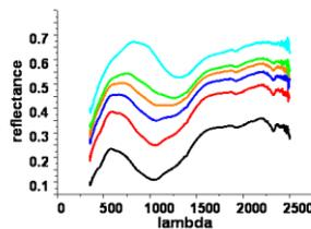
Fig. 4 Ol-rich+ iron-rich PI mixture's reflectance spectra. PI % increases from black to light blue.
