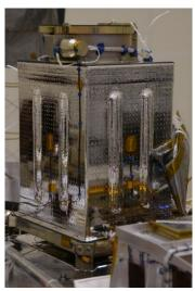
Figure 3: Phoenix Mars Lidar system
