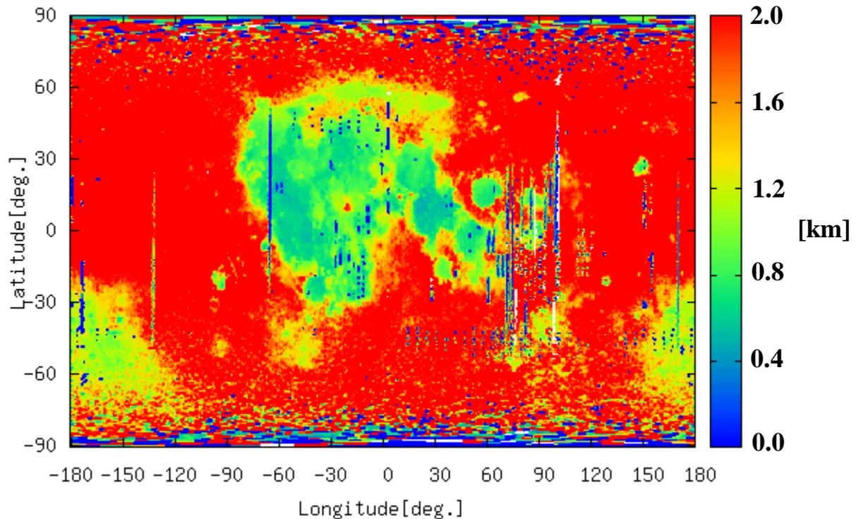
**Fig 1.** Map of Kaguya/LRS maximum detection depth for buried regolith layers with a thickness of 1 m. The maximum detection depth in the nearside maria is about 1km.
