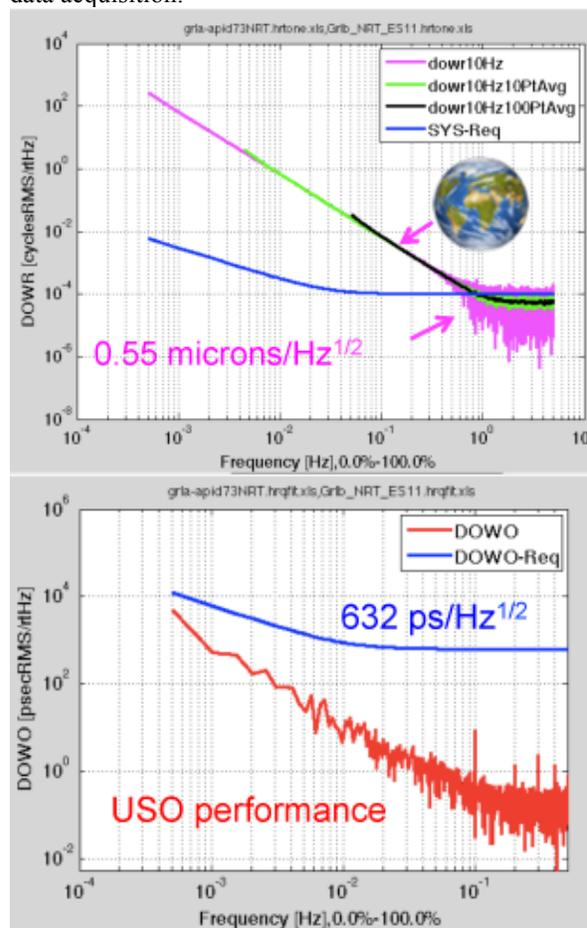
**Figure 2.** Results of GRAIL in-space ranging test, which verified the performance of the mission payload. (Top) Ka-band ranging system performance, plotted as dual one-way range vs. frequency, showing observations (magenta, green black) and requirements (blue). (Bottom) S-band system performance plotted as dual one-way offset vs. frequency. Observed noise (in red) is less than the requirement (in blue) over the full frequency range.
