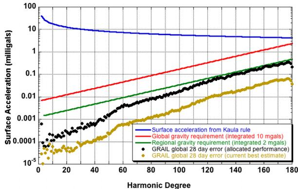
**Figure 1.** Error spectra from simulations illustrating margin between global (red) and regional (green) science requirements and the allocated (black) and current best estimate (gold) of GRAIL's performance. The blue line is the expected surface acceleration spectrum based on an empirical estimation of the power (Kaula's rule) [7] in the Moon's gravitational field.
