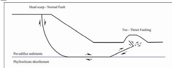
**Figure 4:** Schematic structural interpretation of the Southern EOMBS.
