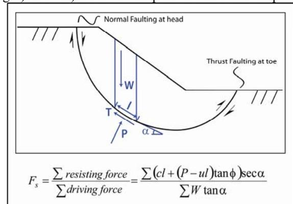
**Figure 3:** Calculating the Factor of Safety (FS) from driving and resisting forces using Janbu's simple method (force balance approach) and circular failure surfaces. Where,  $W$  = slice weight,  $T$  = resisting force acting on a slice,  $\alpha$  = angle from horizontal to failure surface,  $P$  = normal force acting on a slice,  $l$  = length of slice along the failure surface,  $\mu$  = pore fluid pressure,  $c$  = cohesion, and  $\phi$  = angle of internal friction.
