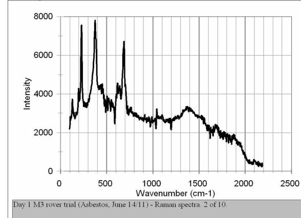
**Fig. 3.** Raman spectrum of an oxidized serpentine from the Jeffrey Mine rover traverse.
