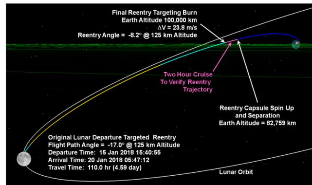
**Figure 2:** MAV return trajectory from the South Pole Aiken Basin.
