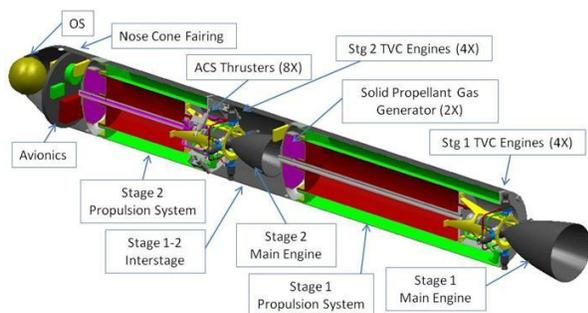
**Figure 1:** The NGAS design for a Mars Ascent Vehicle.
