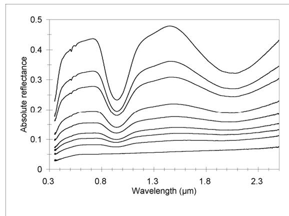
**Fig. 4.** Reflectance spectra of  $<45 \mu\text{m}$  size intimate mixtures of the Millbillillie euclite + the Murchison CM2 chondrite. % Murchison from top to bottom: 0, 5, 10, 20, 30, 40, 50, 60, 100.
