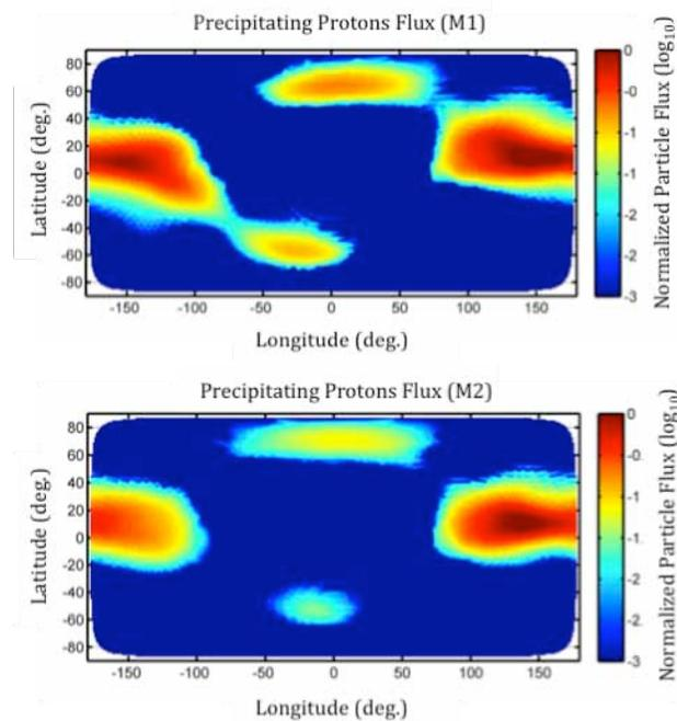
**Fig. 1.** Maps of precipitating proton flux onto the surface of Mercury during the first (M1, top) and second (M2, bottom) MESSENGER flybys modeled from Magnetometer measurements. 0° longitude corresponds to local noon. The fluxes are normalized to the flux of the undisturbed solar wind ( $9 \times 10^8$  particles/cm<sup>2</sup>/s during M1 and  $6 \times 10^8$  particles/cm<sup>2</sup>/s during M2).
