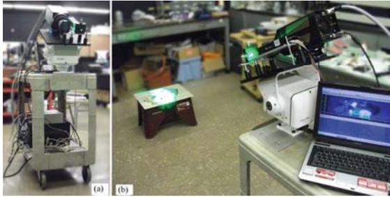
Fig 2: (a) A prototype standoff bio-imaging system utilizing an ICCD camera, a 532 nm pulsed laser (0.1 mJ/pulse) mounted on a portable trolley with a pan and tilt scanner. Fig 2(b) shows the front view of the system in action looking down towards several targets placed at 2 m distance.
