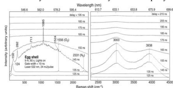
Fig 1. Time-resolved Raman and fluorescence spectra of a chicken eggshell from a distance of 9 m measured with the Univ. of Hawaii's 5-inch stand-off Raman system in gated mode. Delays on the curves are the time in nanoseconds after the Q-switch of the laser is triggered. Laser: 532 nm, 24 mJ/pulse, 20 Hz; gate width 10 ns.
