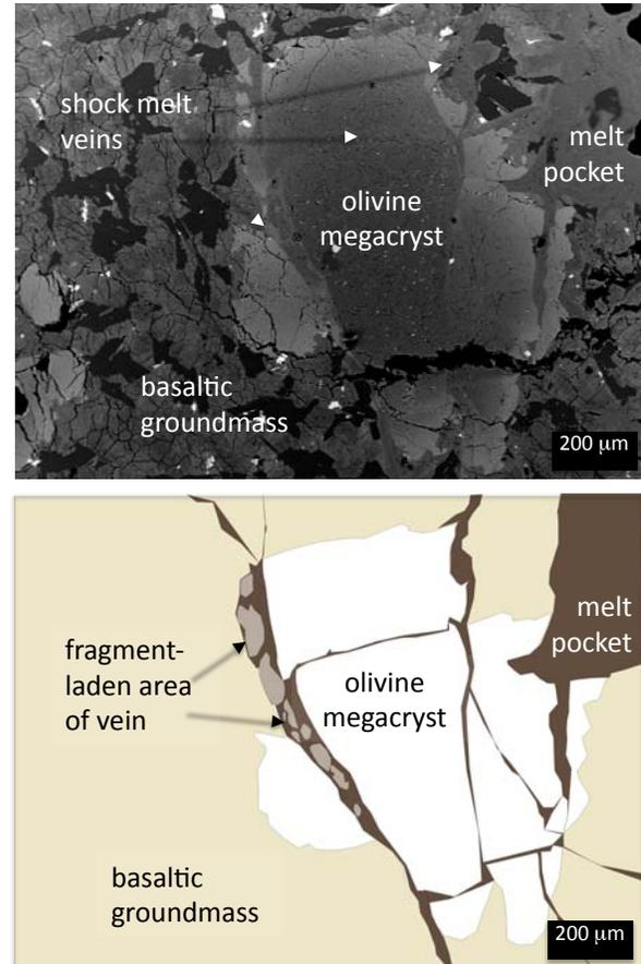
Figure 1. (top) BSE image of zoned olivine megacryst cut across by an interlocking network of shock veins. A sketch of the corresponding area (bottom), shows the relationship between shock melts (brown), basaltic groundmass (yellow) and the olivine megacryst (white).
