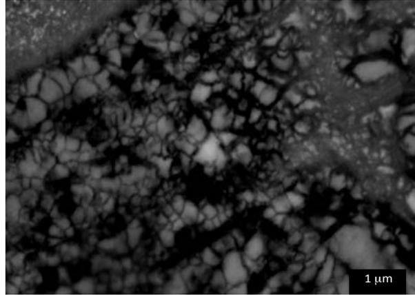
Figure 2. BSE image of polycrystalline ringwoodite aggregates on olivine fragments entrained within the shock vein.
