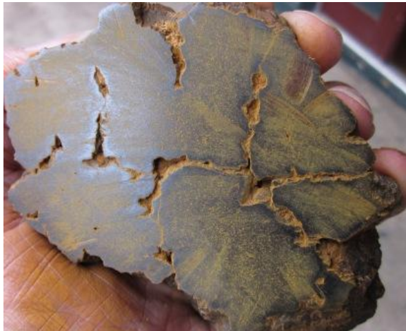
Figure 3. Interior of the mass shown in figure 3. Limonite/Hematite pseudomorphs preserve pyrite crystal structure. Less altered masses of iron-sulfide were mined from a pit closer to the crater's center [3].
