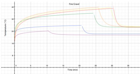
**Figure 1:** Thermal behavior of fine gravel at different levels of saturation: dry (red), saturated within 8 cm below the surface (orange), 6cm below the surface (yellow), 4cm below the surface (green), 2 cm below the surface (blue), and completely saturated (violet).
