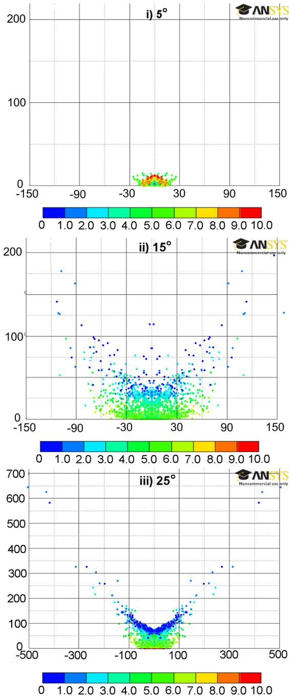
**Fig. 2:** Spatial distribution of projectile fragments on a witness plane 120 micrometres from the projectile impact point for an impact angle of **i)** 5°, **ii)** 15°, **iii)** 25°. Numbers on the axes are perpendicular distances (in micrometres) from the impact point. Colours correspond to absolute velocities at the witness plane position in  $\text{km s}^{-1}$ .
