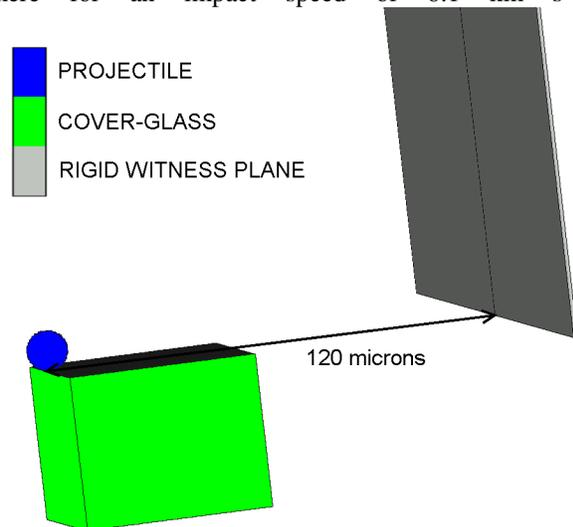
**Fig 1:** Diagram showing the geometry of the model. The grey plane acts as a rigid witness plate.
