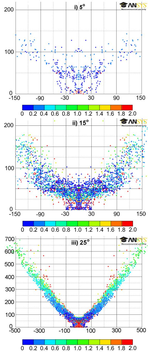
**Fig. 3:** Spatial distribution of target fragments on a witness plane 120 micrometres from the projectile impact point for an impact angle of **i)** 5°, **ii)** 15°, **iii)** 25°. Numbers on the axes are perpendicular distances (in micrometres) from the impact point. Colours correspond to absolute velocities at the witness plane position in  $\text{km s}^{-1}$ .
