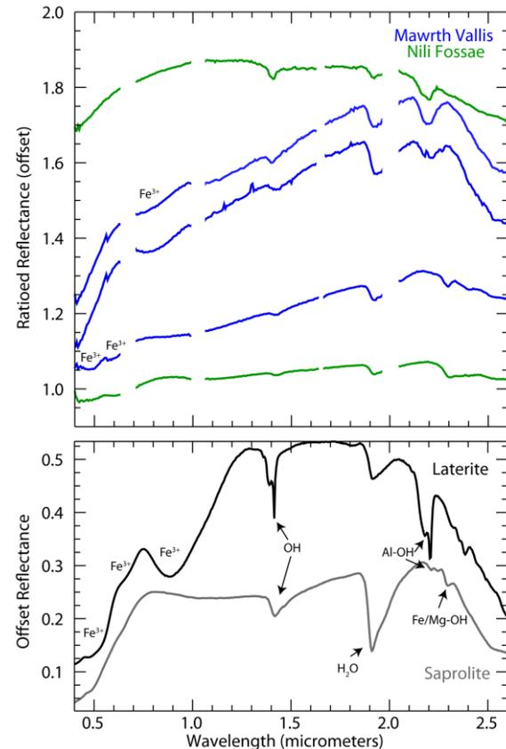
Fig. 2: Example ratioed CRISM spectra (top) from Mawrth Vallis (blue) and Nili Fossae (green). The top three spectra in the top plot are Al phyllosilicates, and the bottom two are Fe/Mg smectite clays. Spectra of two samples from the Deccan analog are shown in the bottom plot for comparison.
