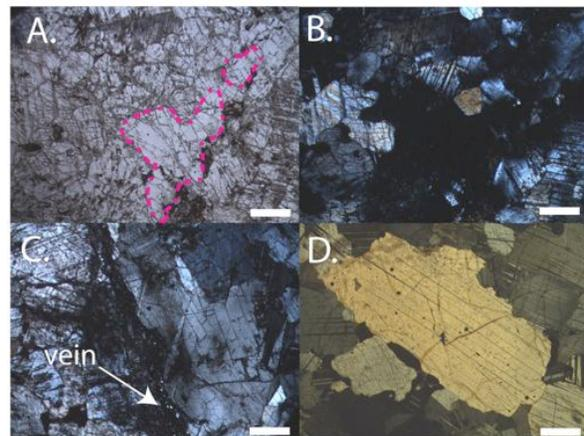
Fig 1: Optical images of plagioclase crystals analyzed. All images taken in cross-polarized light (XPL) with the exception of (A). (A) Shock-fractured plagioclase and maskelynite (traced) in plane-polarized light. (B) XPL view of A, showing isotropic maskelynite. (C) Clast-bearing glassy vein. (D) Unshocked anorthosite crystal. Scale bar is 1000  $\mu\text{m}$ .
